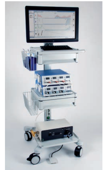
3-channel PeriFlux System 5000 including automatic cuff inflator for measurement at three sites simultaneously.
